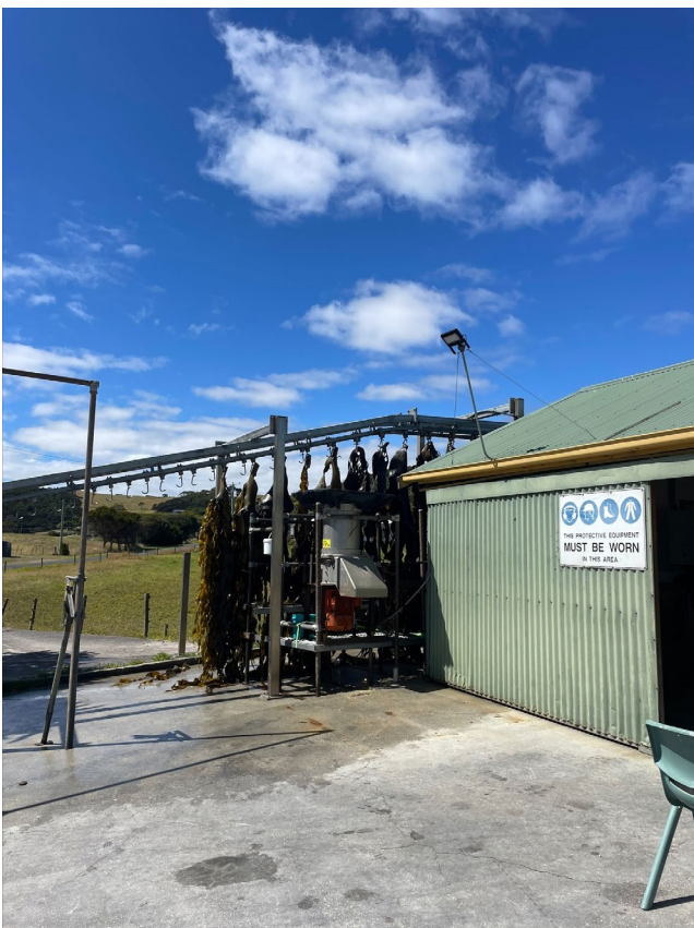
Figure 2: Electric kelp drying rack loaded with bull kelp moving product into the drying shed. Source: Marrawah Gold Pty Ltd
