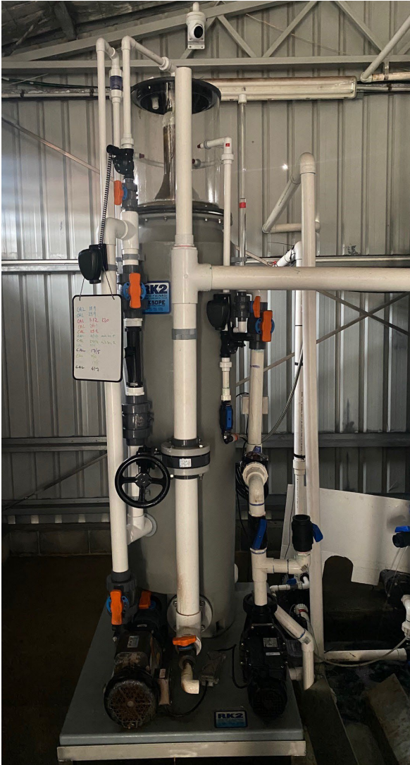
Figure 1: The fractionator—part of the environmental monitoring system, and an example of the real time monitoring out for one of the holding tanks. Source: Seafood Traders Pty Ltd
