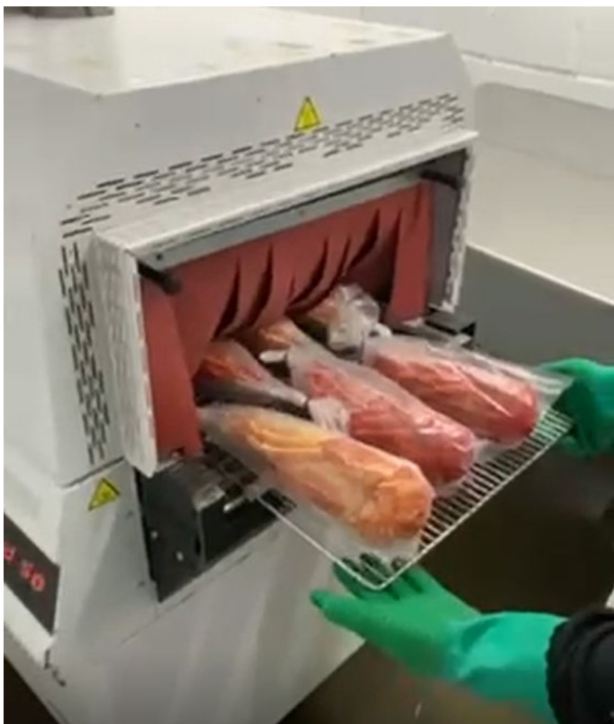
Figure 1: Heat shrink tunnel in operation. Source: Triabunna Lobster Pty Ltd
